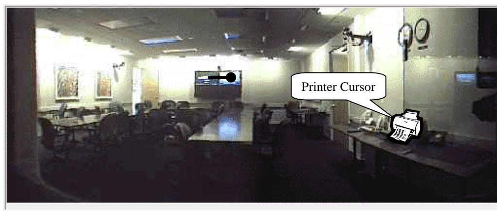
Figure 9. When the mouse cursor moves to the hot spot defined for the printer, it is changed to printer shape.
